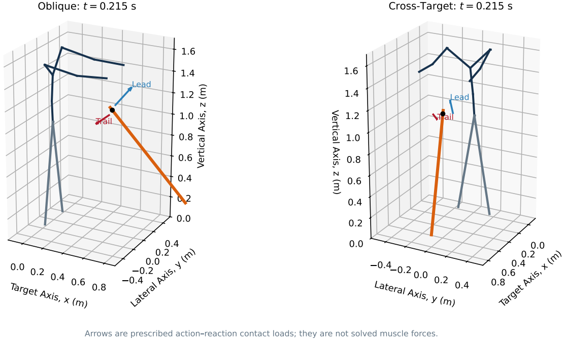
Figure 17.1: Spatial Full-Body Common State and Two-Hand Force Geometry
