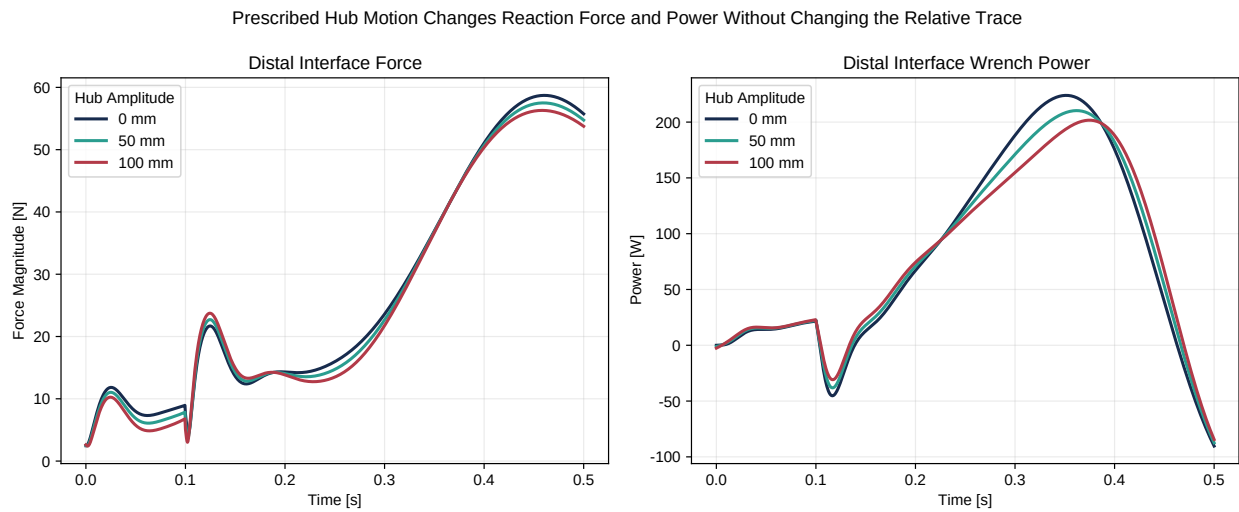
Figure 22.4: Prescribed Hub Motion Changes Reaction Force and Power Without Changing the Relative Trace
